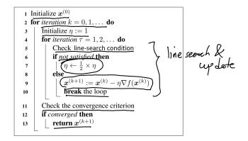
As this algorithm shows, line-search has its own internal iterations inside every iteration of gradient descent.
